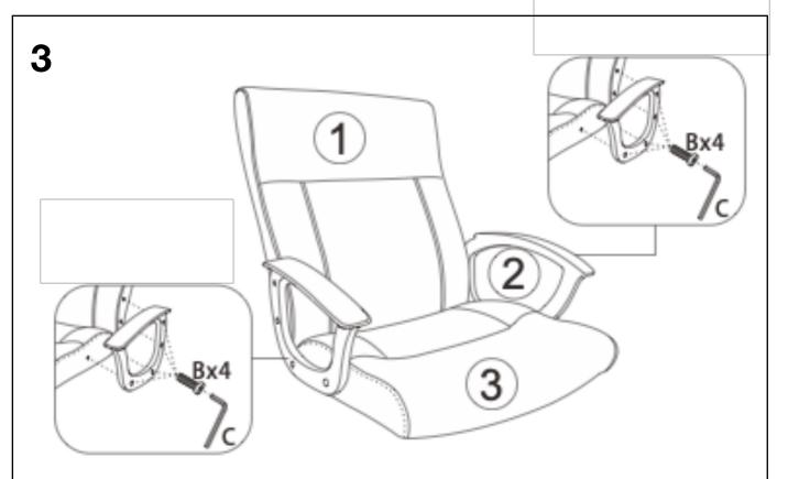
CAUTION: Do not over tighten the bolts, this may damage the product. Tighten only until the thread is firmly in.
