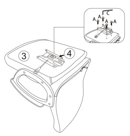
CAUTION: Do not over tighten the bolts, this may damage the product. Tighten only until the thread is firmly in.
